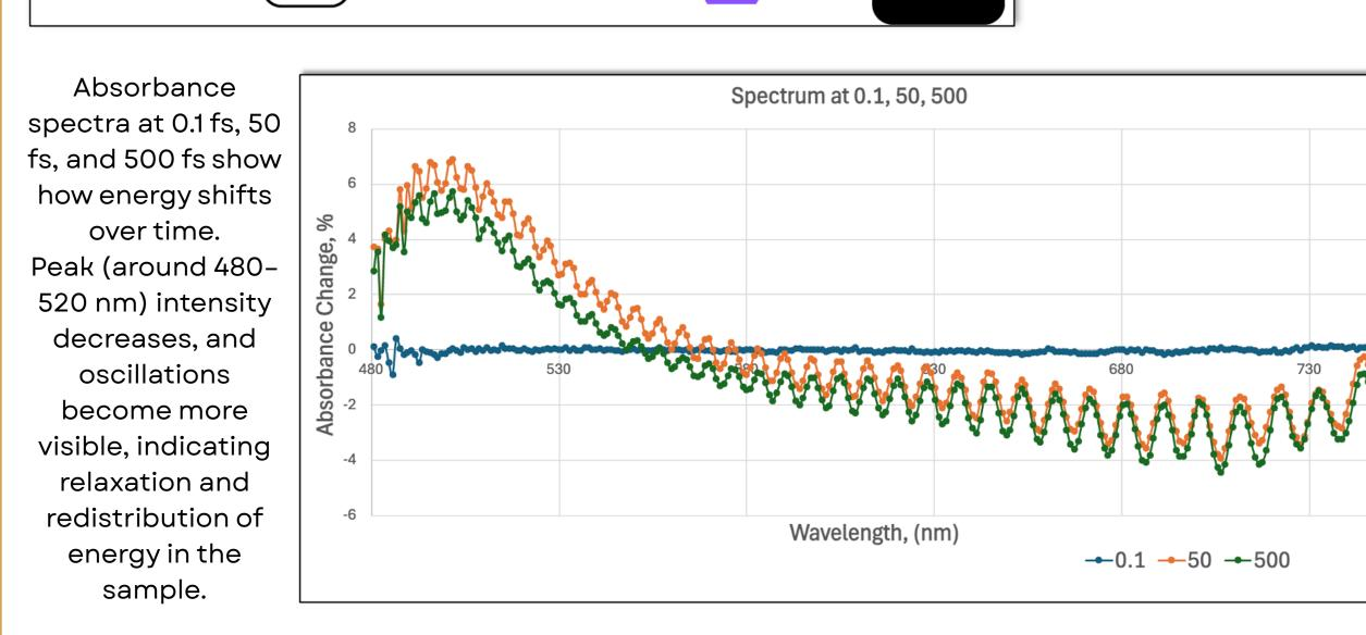
Pump-probe analysis revealed absorbance changes at specific wavelengths, with strong response near 500.79 nm, moderate at 600.19 nm, and minimal at 730.70 nm. These results highlight how ultrafast spectroscopy tracks excited-state dynamics on extremely short timescales.
