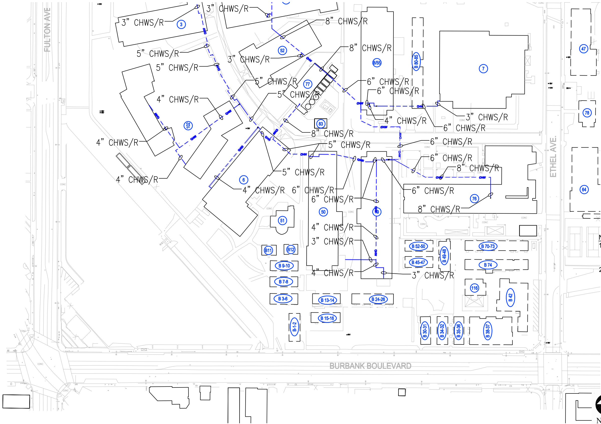
FIGURE 8c EXISTING CONDITIONS UTILITY MAP - CHILLED WATER
