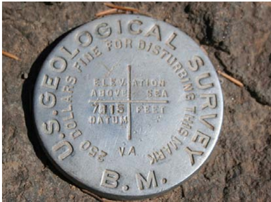
Marker Example: Datum (includes identification information) Material: Engraved Metal
